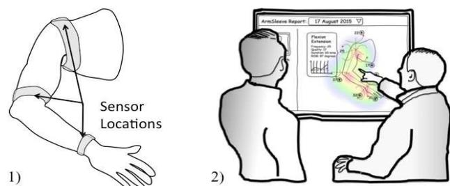
**Figure 1: The ArmSleeve system was designed to support occupational therapists through objective upper limb data captured in the daily life of their patients. The system consists of the (1) ArmSleeve sensor prototype and (2) a dashboard.**
