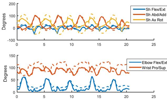
**Figure 3: Comparison of motion data captured from ArmSleeve Sensors (solid lines) and Vicon® Motion Capture System (dashed lines). The graph shows shoulder (top), elbow and wrist motion (bottom) for 5 sets of swinging the right arm.**
