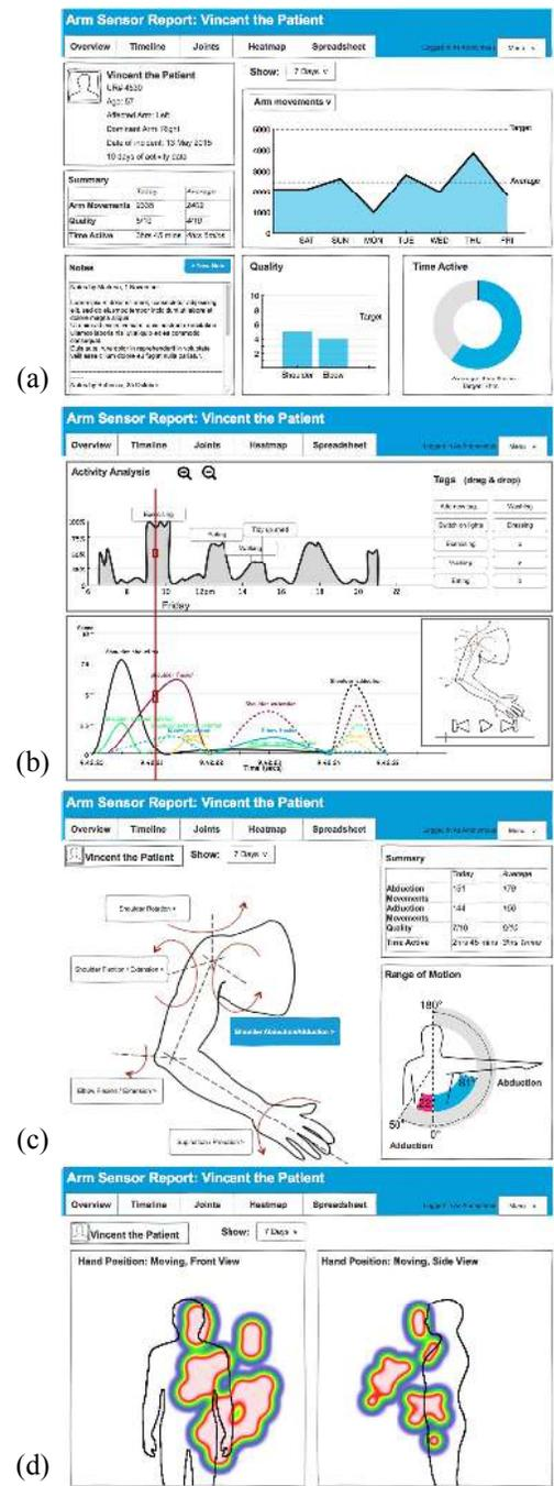
**Figure 4: The ArmSleeve dashboard provides (a) a patient overview page, (b) a timeline with the ability to tag data points, (c) visualizations for range of motion for each joint, and (d) heat maps to show common arm positions.**
